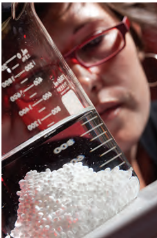
At Yale, recyclable chitosan-titanium dioxide beads are used for sorption of arsenic from contaminated water. [Photo: Harold Shapiro]
