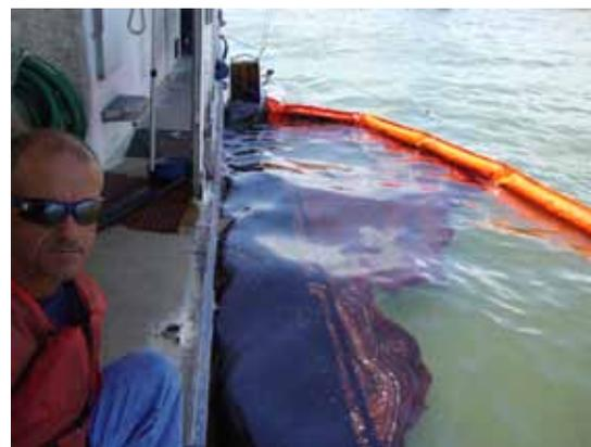
*Polyvinyl chloride (PVC) coated fabric booms manufactured by Connecticut-based Slickbar Products were deployed to contain oil from the massive BP spill. [Photo: Slickbar]*
