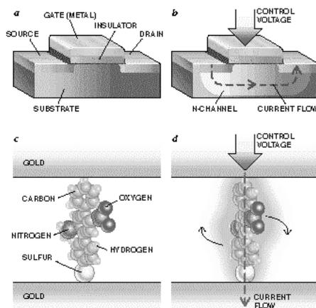
The conduction path in a conventional microelectronics transistor is turned on using an applied voltage at the gate electrode. Similarly, the conduction path through a molecular switch is turned on by an applied voltage. The applied voltage is believed to cause a conformational shift which, in concert with the charging of the molecule, opens the conduction pathway. (Photo: Mark Reed)
